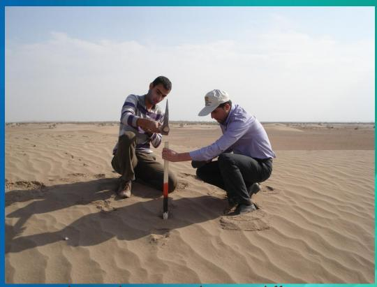
Fixing the wind erosion indexes on different parts
