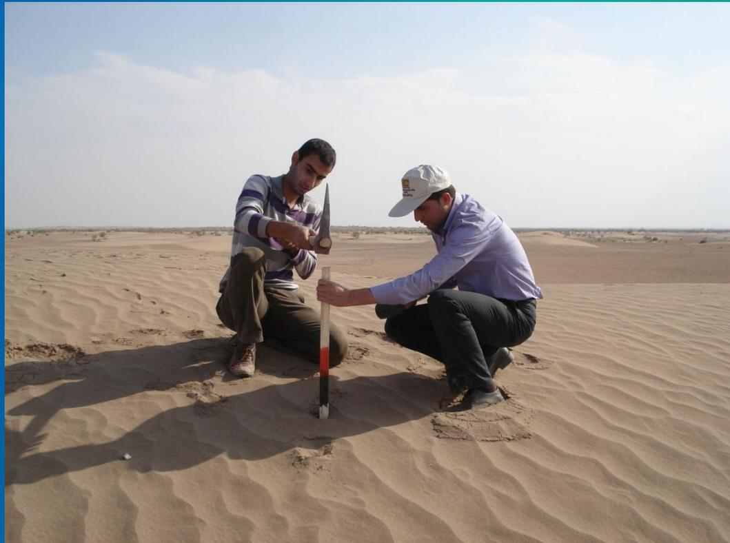
Fixing the wind erosion indexes on different parts
