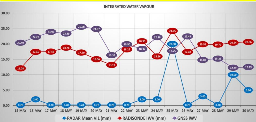
IWV data of GNSS and Radiosonde (00Z and 12Z)
